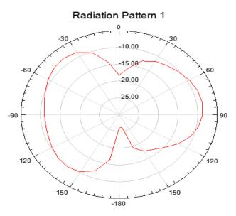
Radiation pattern for proposed antenna with DGS
